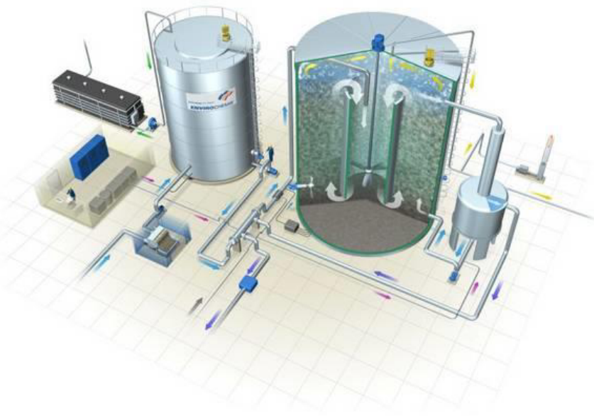
Fig. 3. Biomar ALB: anaerobic method using upflow reactor.
