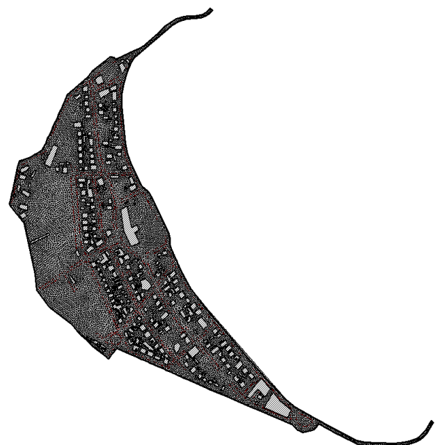
Figure 4. Finite elements mesh of the study area
