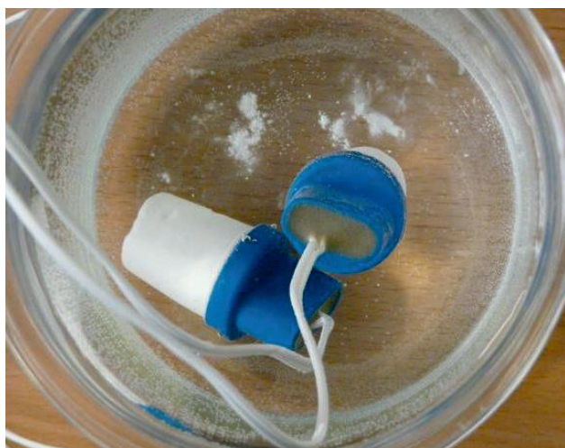
Figure 3. Gypsum blocks used in the first test at the end of their saturation prior to their installation in the sample. Gypsum residue may be clearly seen at the bottom of the glass jar holding the gypsum blocks in deionised water.
