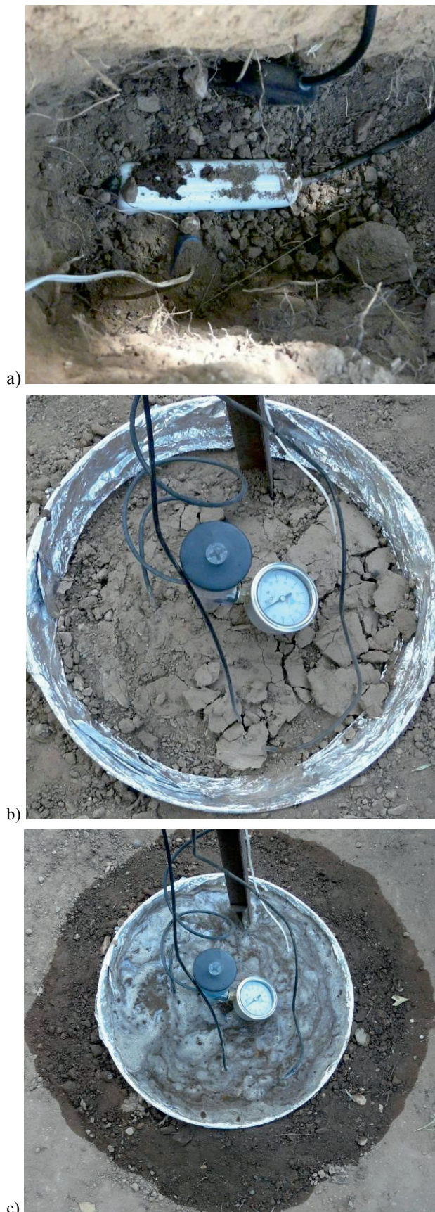
Figure 6. a) Open hole for the installation of the first set of sensors in the Artemida field array (top: MPS-2, middle: GS-3, bottom: Gypsum Block), b) dry surface of the field array before wetting, and c) after wetting (water seeped outside the plastic ring used to contain the free surface of water).
