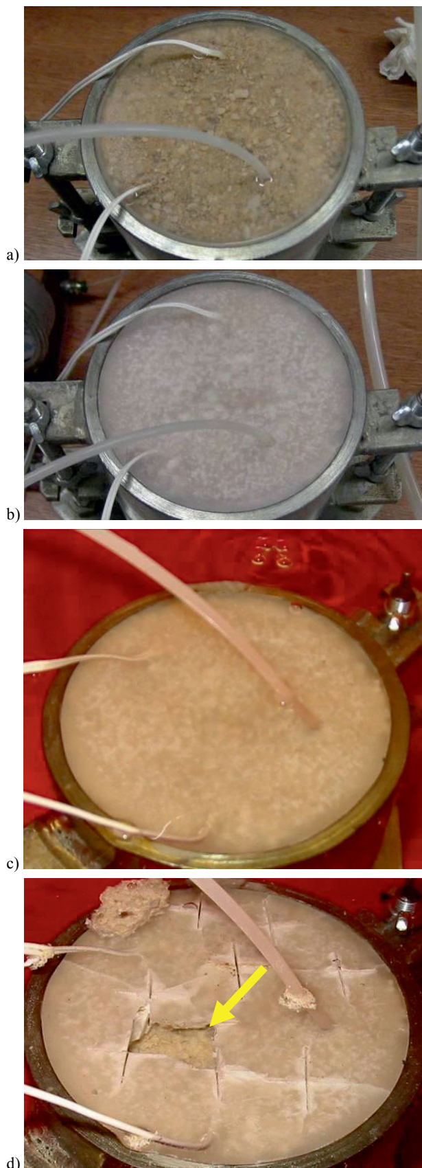
Figure 1. a) Proctor test mould with the paraffin wax immediately after it was poured over the coarse sand, and b) after it set, c) after inundation of the whole mould (bubbles from a tiny hole can be seen), and d) after the wax layer was cut and partially removed (settlement of the sand pointed by arrow).
