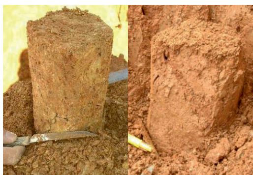
Figure 3. Close view of GrSp soil (left) and GrLt (right).
