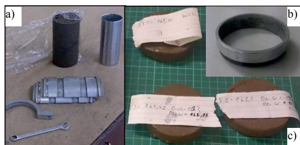
Figure 2. Sample preparation and trimming to desired size: a) sample core extruded after Proctor test; b) stainless still ring; c) soil specimens, size of 20/75 mm.
