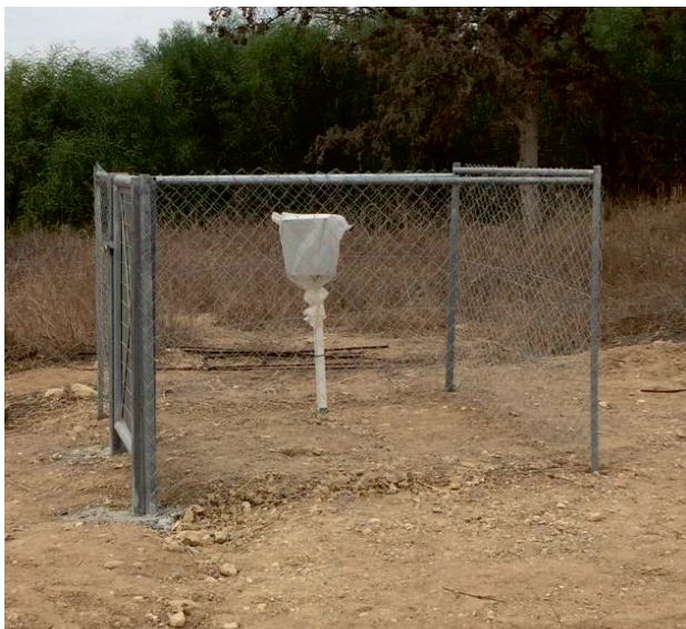
Figure 4. Trial pit backfilled and fenced to protect the sensor data acquisition box.
