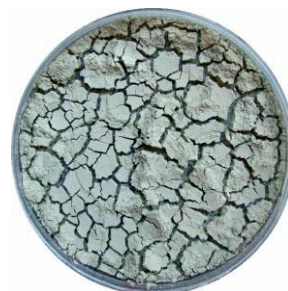
Figure 7. The crack pattern after the second wetting-drying cycle.
