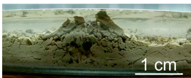
Figure 6. The entrapped air bubble inside the soil during wetting cycle
