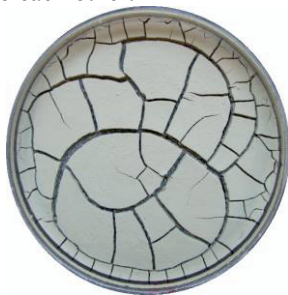
Figure 3. The crack pattern after the first wetting-drying cycle.
