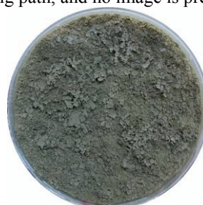
Figure 8. The typical crack pattern during the third wetting path (after about 1 min wetting).
