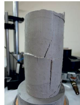
Figure 15. Creep failure of bentonite with water content of 6.80 % at vertical stress of 9.9 kPa.
