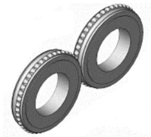
Figure 2. Asymmetrical layout compacting system of laboratory roll press LPW 450
