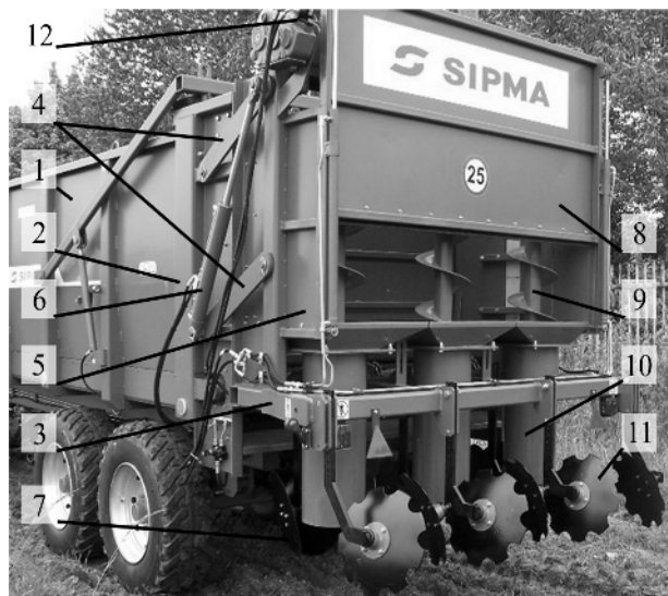
Figure 2. Prototype of device for subsurface application of loose organic and mineral fertilisers manufactured by SIPMA S.A.: 1 - trailer, 2 - base frame, 3 - beam, 4 - arms, 5 – loading chamber, 6 - hydraulic cylinder, 7 – disc coulters, 8 – flap, 9 - screw conveyor, 10 – cylindrical housing of screw conveyor, 11 – ridging plough, 12 – hydraulic engine.
