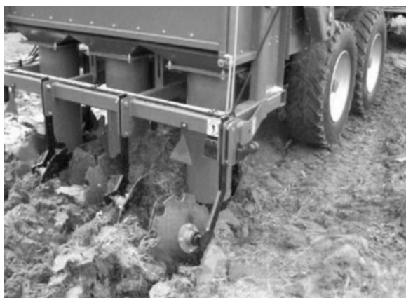
Figure 3. Application of sewage sludge into the soil subsurface.
