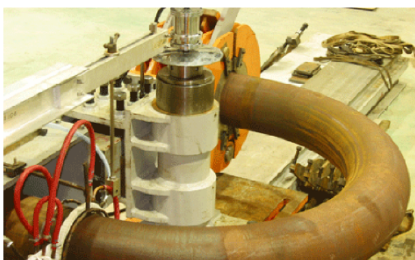
Figure 14. CNC plasma cutting/Flame cutting - High frequency bending and welding.
