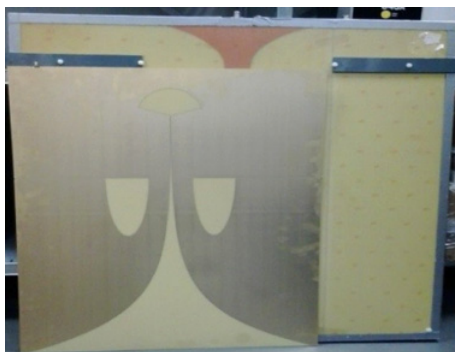
Figure 2. New miniaturized ETSA (Exponentially Tapered Slot Antenna) superimposed on original larger ETSA. The exponential taper (a horn-shape) is clearly visible at the bottom of the figure.
