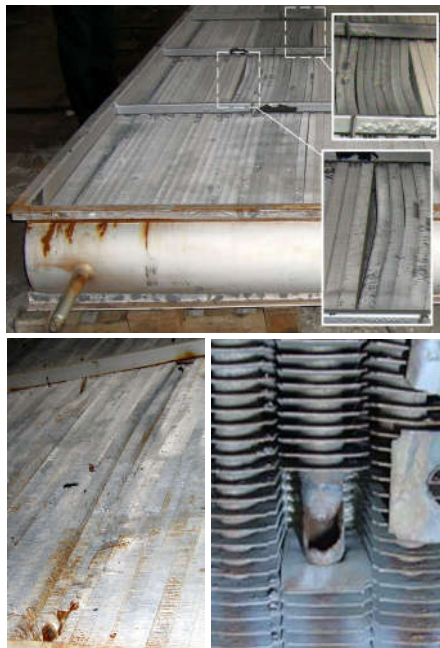
Fig. 3. Buckling and fracture of heat exchanger tubes
