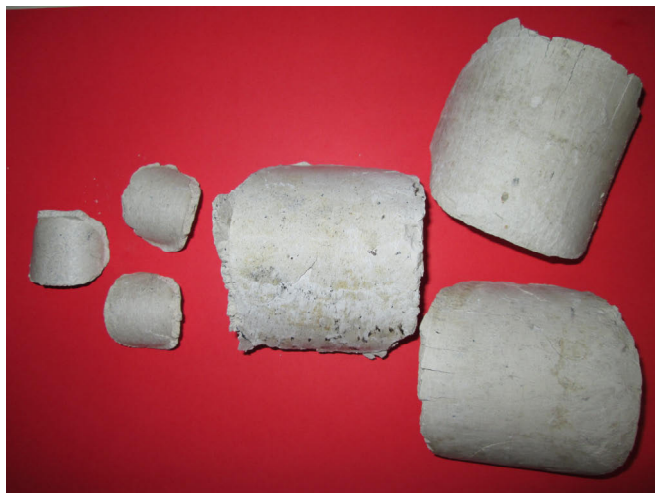
Fig.10. FGD gypsum from Bełchatów power plants briquettes produced in roll press LPW 450 (volume-6,5 cm 3 ) and LPW 1100 (volume-85 cm 3 ).
