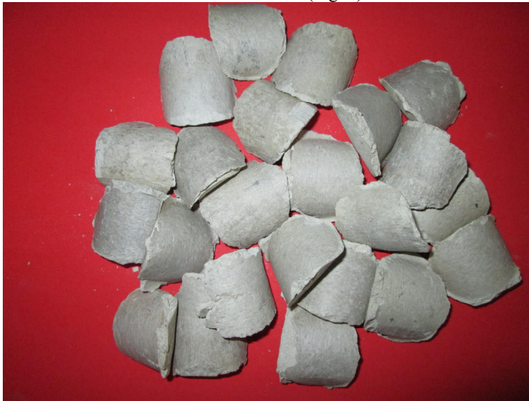
Fig. 3. FGD gypsum from Połaniec power plants briquettes (volume-6,5 cm 3 ) produced in roll press.
