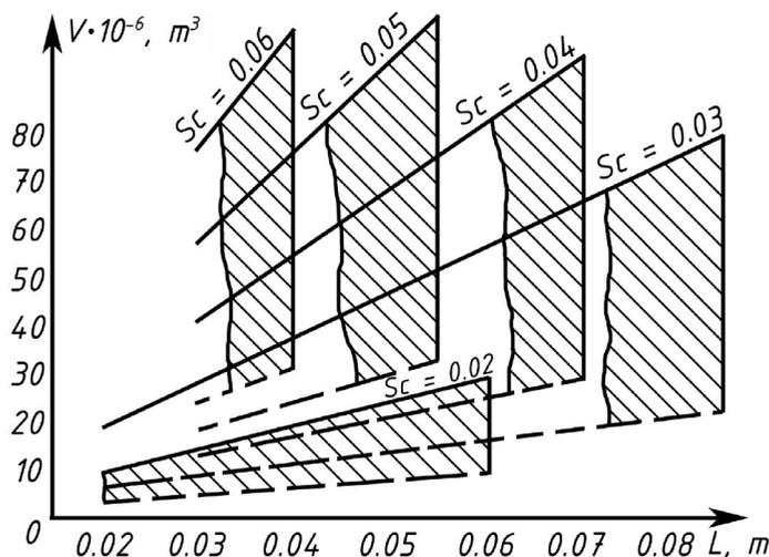
**Fig. 4.** Dependence of the volume of destroyed element ( $V$ ) in one phase of cutting cycle on the height of exposure ( $L$ )
