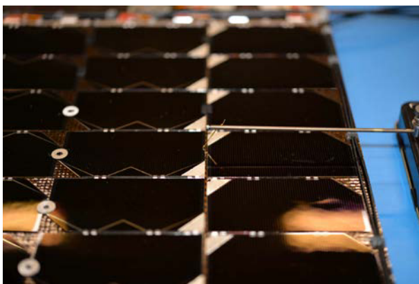
Figure 11. Application of a measurement probe on top of the outer edge of the coverglass. The other electrical connection is done via the grounding bar on the left side (not visible in this picture).
