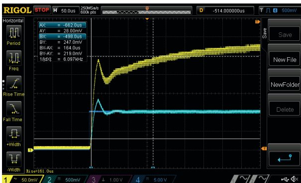
Figure 11. Output voltage of a TMR current sensor under an 7.5A input current step. CH1: TMR output voltage, CH2: Agilent TCP202 Hall current probe output response, CH4: Step control voltage.
