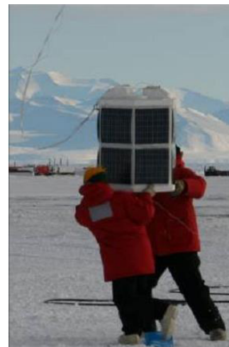
Figure 1: Concordiasi avionic gondola with cuts solar cells
