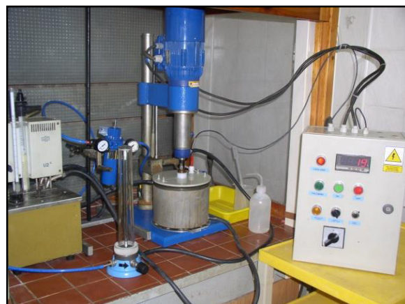
Fig. 1. Laboratory setup for investigation on regeneration of acidic copper chloride solutions.
