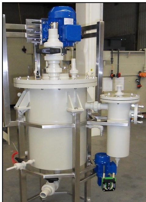
Fig. 2. Reactor of 50 dm 3 volume used for regeneration of acidic copper chloride solutions.
