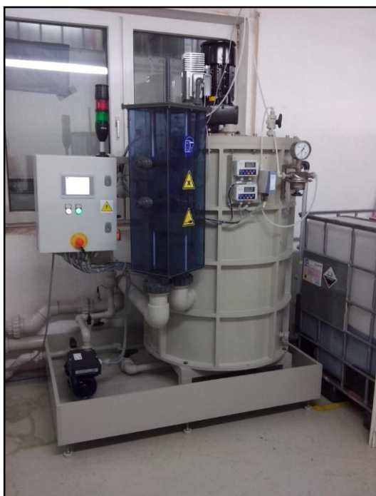
Fig. 4. The technical scale reactor for acidic copper chloride solutions regeneration.
