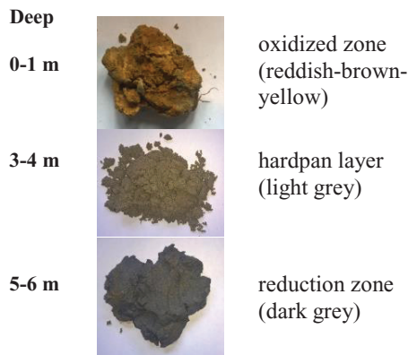
Fig. 2. The colours for oxidation zone, hardpan layer and reduction zone for H3 drill.
