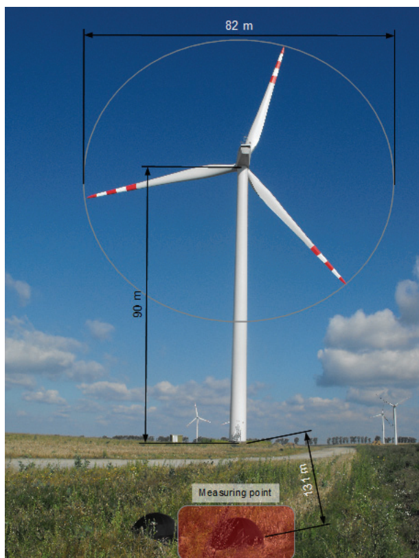
Fig. 1. Location of the infrasound noise level measuring point at the asynchronous type turbine.
