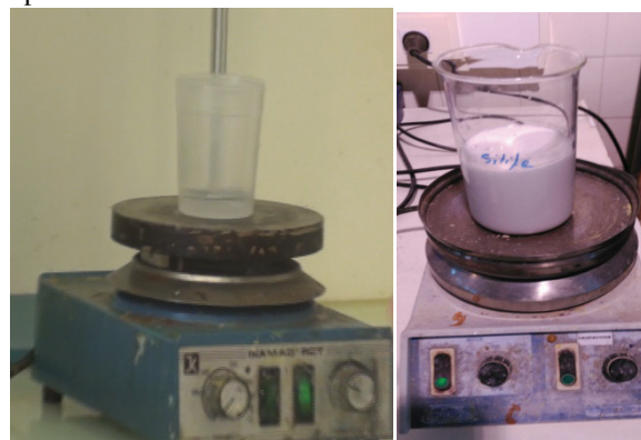
Fig. 3. Hydrolysis with HCl (left). Stirring suspension with quartz (right).
