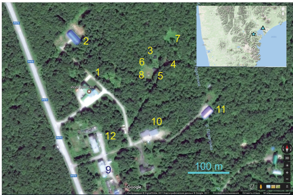
Figure 1. The location of the main buildings and objects near Observatory (from www.google.ru/maps/ ). 1 – main building of institute; 2 – building of ionospheric station (working and office rooms, lidar, ionosonde Parus with vertical dipole transmitting antenna oriented in SE-NW direction); 3 - pavilion for variation measurements (magnetometers FGE, GSM-90, MAGDAS, FRG-601); 4 – pavilion for absolute observations (magnetometers LEMI-203, Mag-01H, POS-1); 5 – technical pavilion; 6 – pavilion for magnetometer dIdD GSM-19FD; 7 – sensors of induction magnetometer STELAB; 8 – area with electric field meter Pole-2; 9 – azimuthal target at wall of house, the its visibility from absolute pavilion is provided by glade; 10 – garage and workshops; 11 – service building; 12 – two three-store buildings. The POS-4 pavilion is placed between pavilions 3 and 4. At the left of photo there is federal road between Paratunka and Petropavlovsk-Kamchatsky. The framing shows the map of central part of Kamchatka with Petropavlovsk-Kamchatsky (▲) and Paratunka (★).
