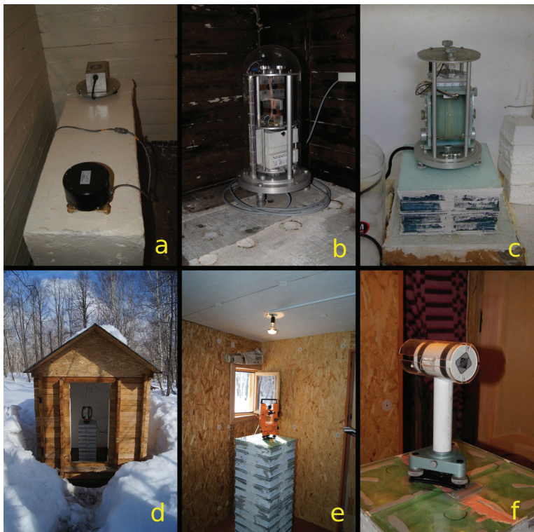
Figure 3. Magnetometers of the Observatory Paratunka: (a) the sensors of the fluxgate magnetometers Magdas (in front) and FRG-601 (at the back) in the variation pavilion; (b) - the suspended sensor block of the fluxgate magnetometer FGE in the variation pavilion; (c) – sensor of magnetometer diD GSM-19FD on a low pillar in a special pavilion; (d) - pavilion of the magnetometer POS-4 with a sensor on the pillar; (e) - Diflux LEMI-203 on the main pillar in the absolute pavilion with the window to observe the remote target (at the back); (f) – sensor of magnetometer POS-1 on the main pillar in the absolute pavilion.
