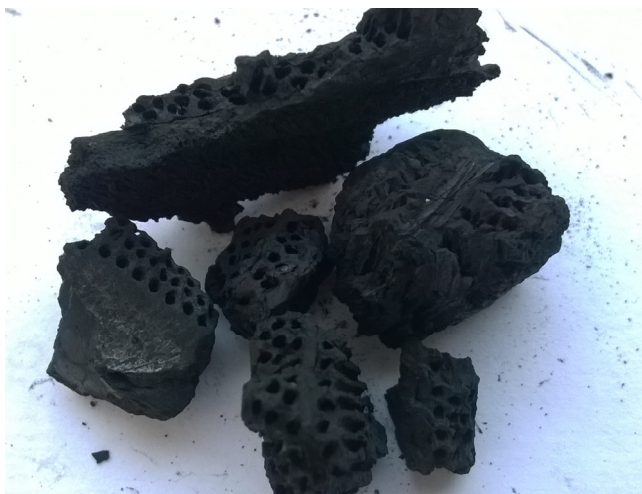
Fig. 2. Carbon residue of tire pyrolysis upgraded by heat treatment
