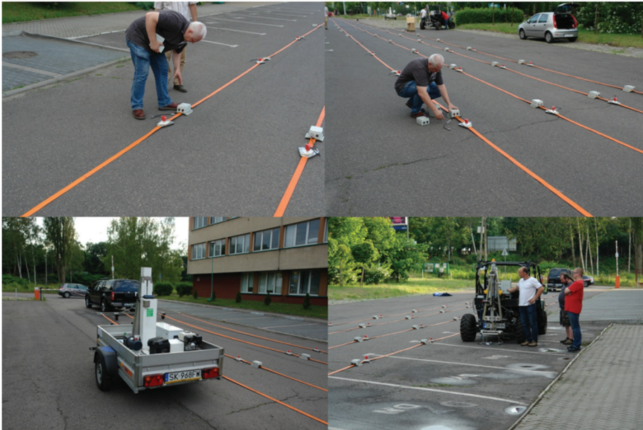
Fig. 2. Preparation of the measuring set for Seismobile testing (assembly of sensors and measuring modules on the tape of S4 streamer), and excitation of a seismic wave signal using the 90-kg pile-driver (trailer) and the 45-kg pile-driver mounted to the KAWASAKI mini car.
