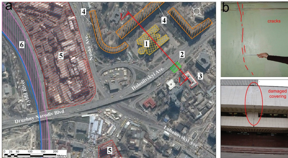
Fig. 1. The plan of the experimental site (a) and the damage on the constructions of building (b): 1 – the building of the library; 2 – the metro station; 3 – the school; 4 – residential buildings; 5 – industrial enterprises; 6 – railway tracks.
