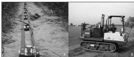
Fig. 1. In section A – part of projected land streamer, B – seismic source used for surveys.
