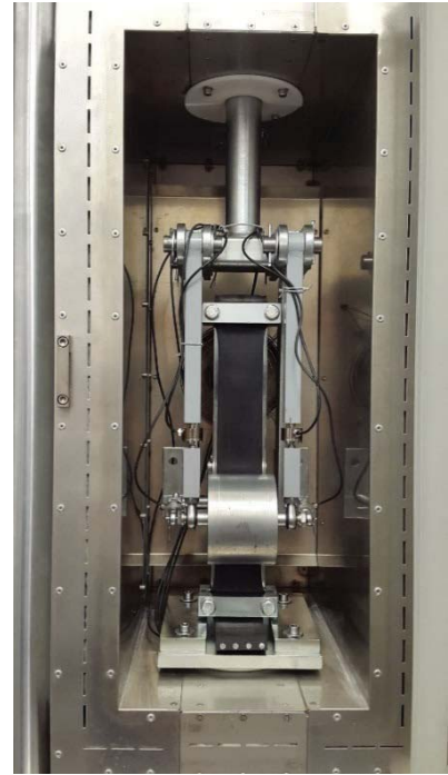
Fig. 3. Test rig for measuring indentation rolling resistances in a thermal chamber (PWr) [12].
