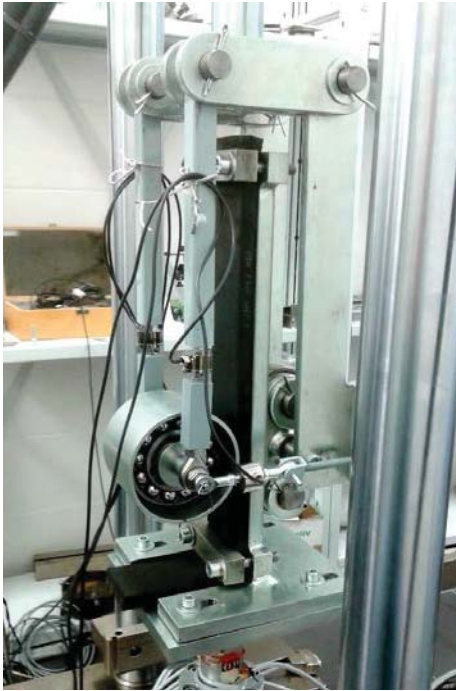
Fig. 2. Test rig for measuring indentation rolling resistances (PWr) [12].
