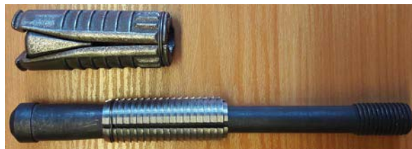
Fig. 3. Expansion shell; upper with diameter 0.036 m equipped with three jaws for bolt with a length 1.8 m, lower with diameter 0.0254 m equipped with four jaws for bolt with a length 3.6 m and 5.2 m (photo: K. Skrzypkowski).
