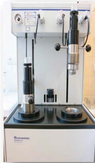
Fig. 2. Porosimeter AutoPore IV 9520 (Micromeritics) [7 , modified].
