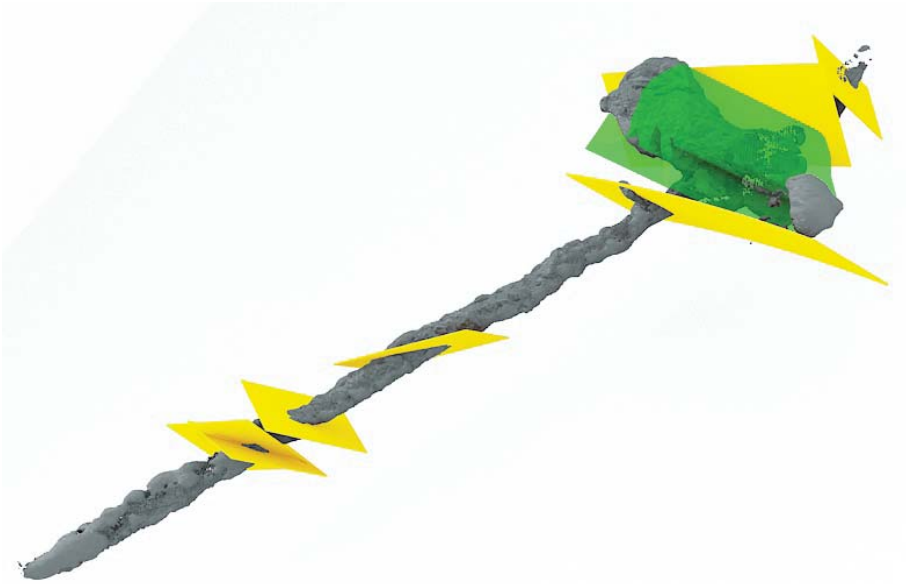
Fig. 7. 3D geological model of the surveyed area: adit (grey), faults (yellow) and body of crystalline limestone (green).
