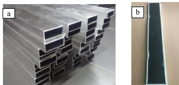
Fig. 1. Aluminium rectangular tube: a-empty, b-filled with PCM and prepared for experimental study
