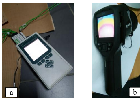
Fig. 5. Data logger (a) and thermal imaging camera (b)
