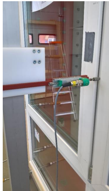
Fig. 5. Linear displacement detectors to determine the relative deflection of mullions
