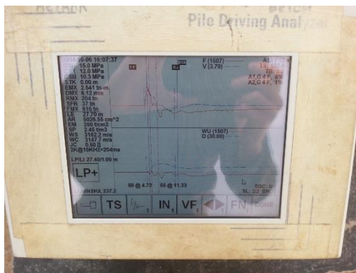
Fig. 8. Computer monitor recording the ELDY test process of pile No. 237.
