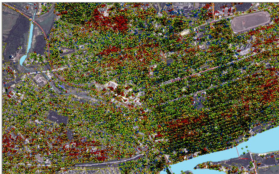
Fig. 4. Pockets of vertical offsets of the city of Rostov-on-Don, obtained on the basis of data of interferometric photography. Red dots indicate significant subsidence of the earth's surface
