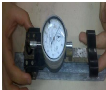
b) Measuring shrinkage using demec gauge.
