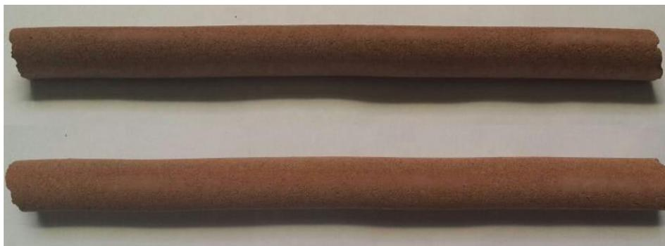
**Fig. 1.** A photograph of porous tubular ceramic supports.
