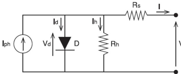
**Fig. 1:** Electrical model of a PV panel.
