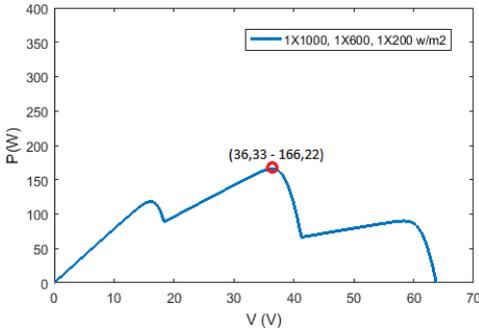
**Fig. 7a:** Characteristic (P-V) at different illuminations in the presence of bypass diode.
