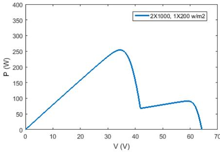
**Fig. 6a:** P-V Characteristics of three PV cells with different irradiance with bypass diode.
