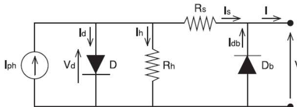
**Fig. 2:** Electrical model of a PV panel with bypass diode  $D_b$  [2].
