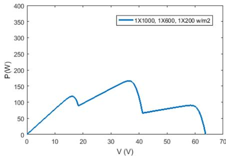
**Fig. 6c:** P-V Characteristics of three PV cells with different irradiance with bypass diode.
