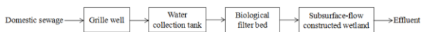
Fig.2-1. The flow chart of the pilot project of the biological filter and subsurface-flow constructed wetland coupling process
