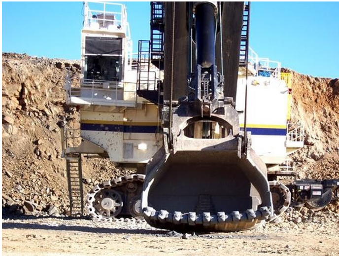
Fig. 1. The shape of the Bucyrus 495HD excavator bucket.
