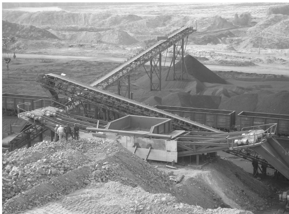
Fig. 1. Design of a DSKA complex, capacity 1500 t/h; Pereyaslavsky open pit mine, Krasnoyarsk.
