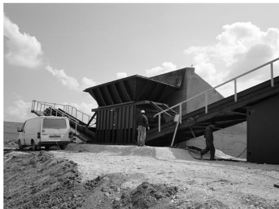
Fig. 4. Design of a DSKA complex, capacity 600 t/h, for one-stage crushing (to 0–25 mm size) and classification of lignite, Pelister Bitola, Macedonia,
