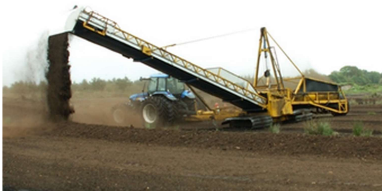
Fig. 3. Peat harvesting by windrowing machines (Bord na Mona, Ireland).
