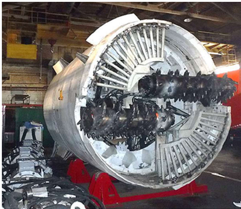
Fig. 1. A Pilot Model of the geokhod with Drum Executive Body (EB).
