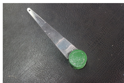
Fig. 7. Pendulum with mass 20 gram and arm length 106.7 mm.
