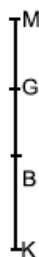
Fig. 8. Position points for positive stable objects (K = keel, B = COB, G = COG, and M = metacenter)
