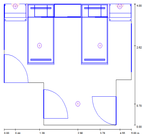
Fig.6. Fixture placement in optimum condition.
