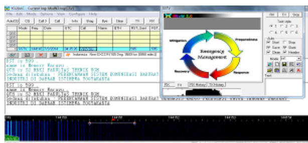
Fig. 8. The image data before it is sent using MixW 3.11g in the mode of SSTV
