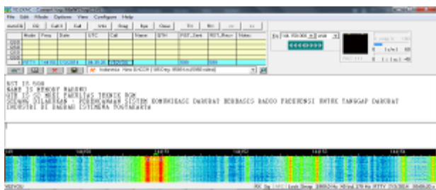
Fig. 6. The process of receiving text data using MixW 3.11g in the mode of RTTY (maximum signal power)
