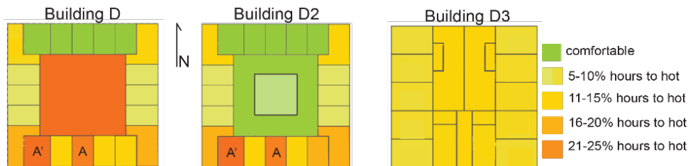
Fig. 6. Selected (4 th floor) layouts of buildings D, D2, D3. Colours indicate percentage of time during the year, when zones are overheated.
