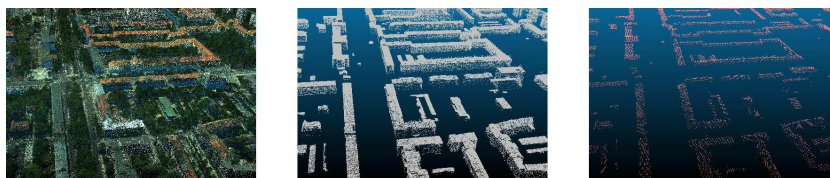
Fig. 2. Points cloud: with RGB mask, selected building class and highest points of rooftop.
