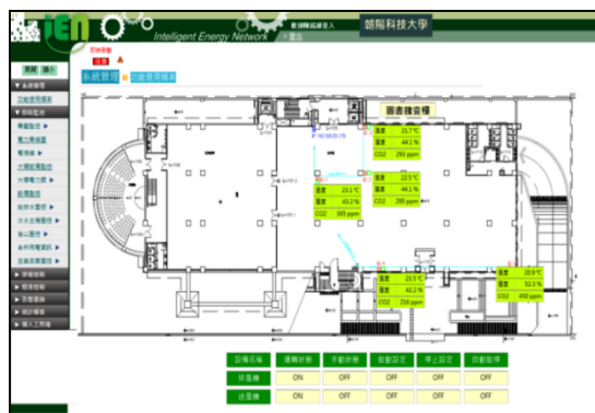
Fig. 5. The control interface of the iEN management and monitoring system in CYUT.
