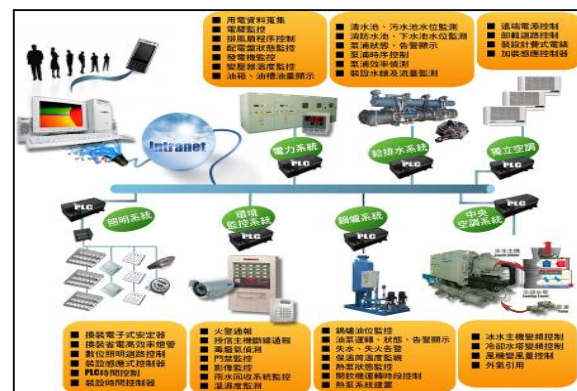
Fig. 4. The framework of the iEN management and monitoring system in CYUT.
