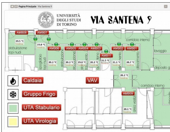
Fig. 5. A screenshot from the building energy management system
